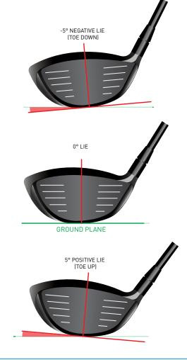
The dynamic measurement in degrees of the club head's face plane position vertically relative to the ground plane. Also known as pitch.
